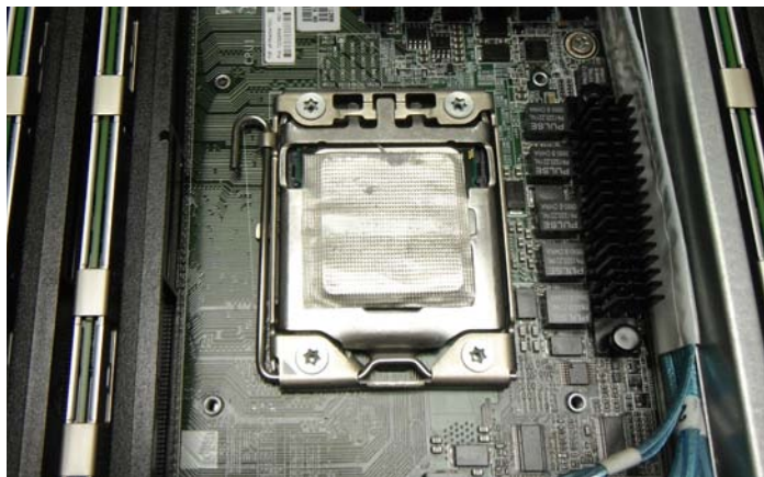
CPU with Indium foil thermal grease substitute
