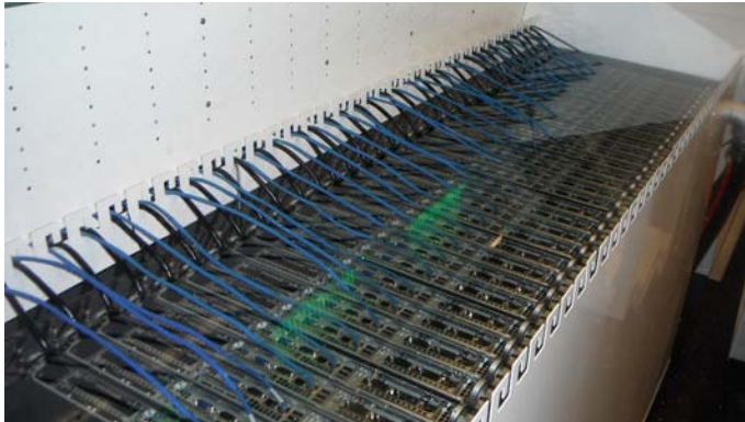
[LEFT]: 42U Rack filled with GREENDEF™ dielectric fluid and OEM servers, [RIGHT]: Four CARNOTJET™ system Racks
