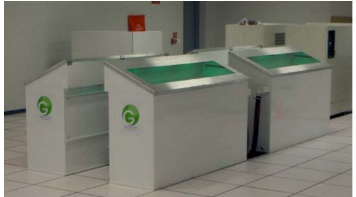
[LEFT]: 42U Rack filled with GREENDEF™ dielectric fluid and OEM servers, [RIGHT]: Four CARNOTJET™ system Racks
