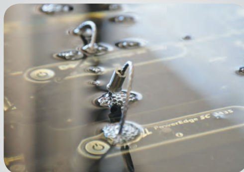
Servers submerged in GreenDEF™ coolant
