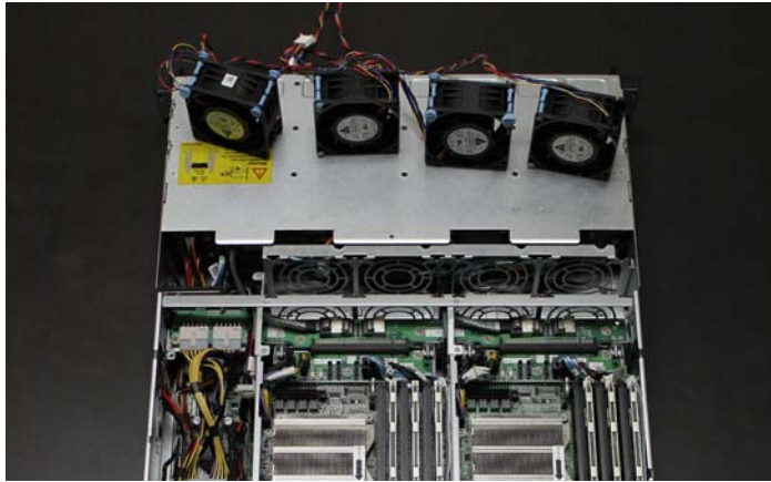
Server chassis fans removed
