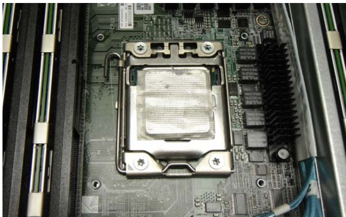
CPU with Indium foil thermal grease substitute
