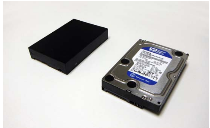
Sealed hard drive [left] and unsealed hard drive [right]
