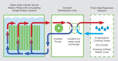
Heated coolant exits top of rack. Coolant returns to rack from heat exchanger at user-specified temperature.
