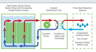
Heated coolant exits top of rack. Coolant returns to rack from heat exchanger at user-specified temperature. ElectroSafe coolants are clean, odorless, nontoxic fluids with 1,200X the heat retention capacity of air by volume. ElectroSafe does not evaporate, resulting in zero Global Warming Potential (GWP).
