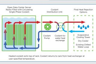
ElectroSafe coolants are clean, odorless, nontoxic fluids with 1,200X the heat retention capacity of air by volume. ElectroSafe does not evaporate, resulting in zero Global Warming Potential (GWP).
