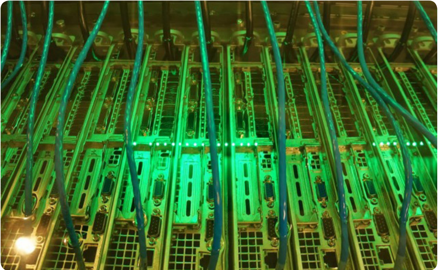
Network servers are submerged into a tank of mineral oil. (Photo used with permission from Green Revolution Cooling: grcooling.com .)
