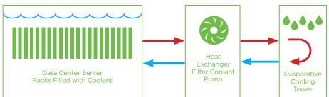
Immersing servers in liquid enables cooling up to 100kW/rack, as liquid has 1,200X the heat retention capacity of air by volume.
